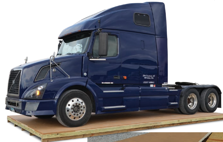
This double 3/4" T&G SmartFloor with standard 16" OC joists on edge shows no deflection from a semi truck's weight. We don't expect you to park a semi truck on a wood floor, but you could!
